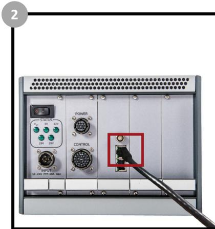
2 Connect the other end of the ethernet cable to the rear of the controller box.
