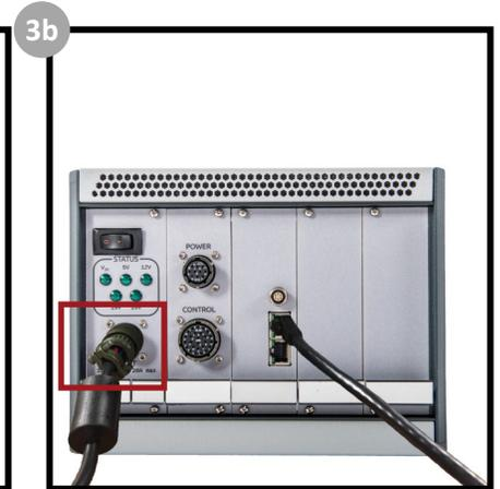
3b Plug the input cord into the rear of the controller box.
