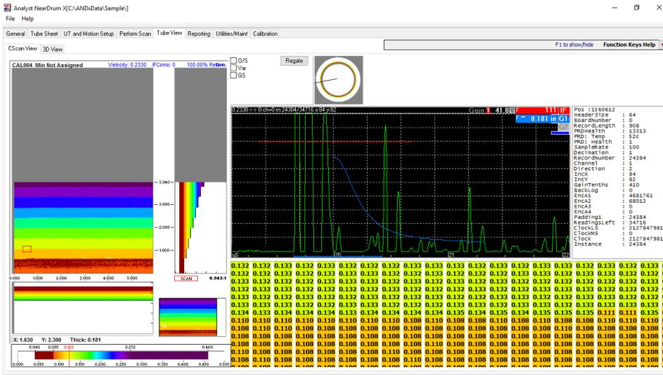
9 Next move to the “Tube View” tab. On this tab, you can re-gate the data, adjust the colormap, or see a 3D view of the tube.
