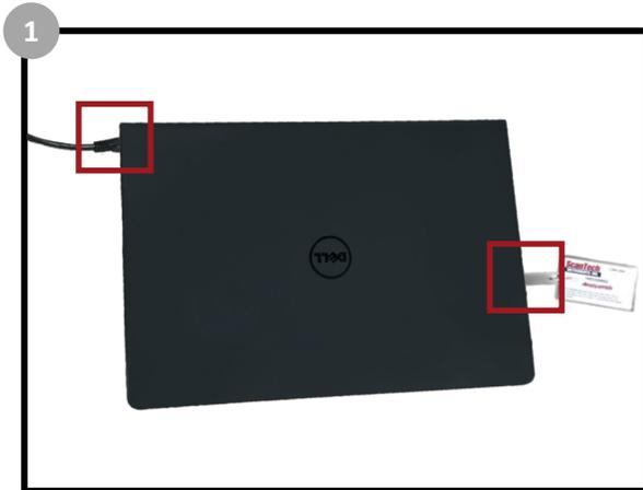
1 Connect the laptop to the controller box using the ethernet cable, and plug in the software key. Turn on the computer.
