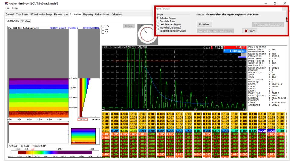
10 Optional: To re-gate the data, click the “Regate” button in the top right corner. Select which region to re-gate, move the gate to the new position, and click “perform regate to these settings”.
