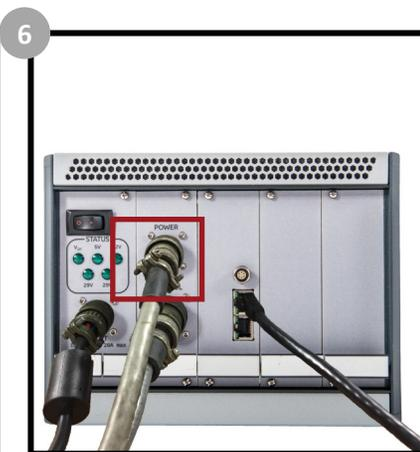
6 Connect the power cable (#3 - refer to the main cable assembly diagram) to the rear of the controller box.
