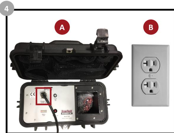
4 If you used cable A: plug the other end of the input cord into the BPS. If you used cable B: plug the other end of the input cord into a wall socket.
