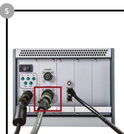
5 Connect the control cable (#2 - refer to the main cable assembly diagram) to the rear of the controller box.
